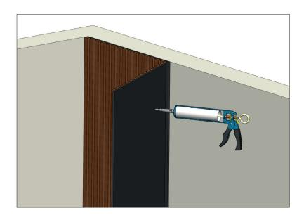
If you choose gluing, you get completely hidden mounting. Our fast-curing glue does it easy to glue the panels. Start always to glue on the panel.
