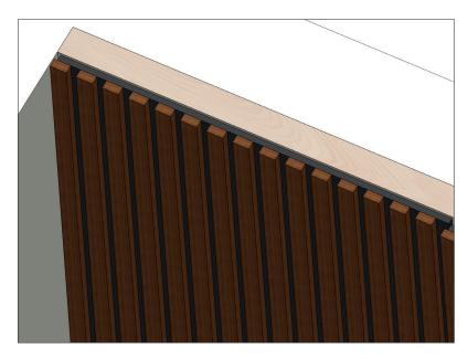
Screw up the panels on the wooden rule. 15 screw/panel.
