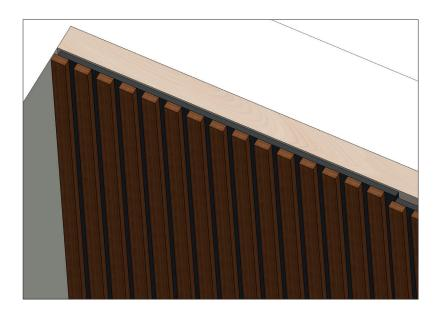
On one side of the panels goes one wooden slats over the edge. It is there to hide the joint.
