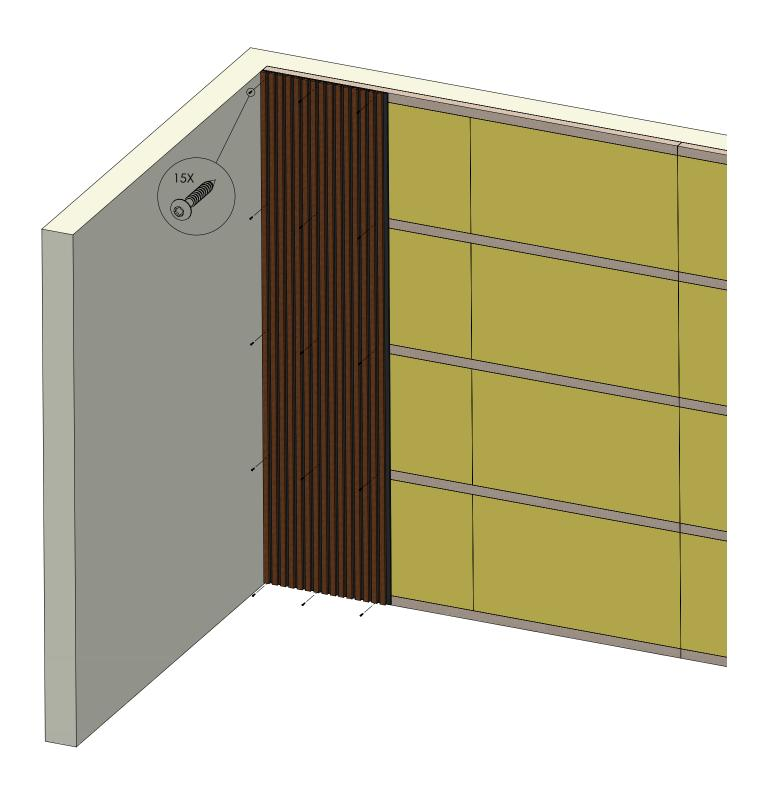
There are different ways to mount Ribbon-Wood. You can screw or glue the panels on existing walls / ceilings. If you want even better acoustics in the room, you can unbolt 45x45mm wooden rule and set insulation (45mm) in between, then you achieve sound class A.
