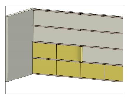
Start to unbolt the wall with 45x45mm wooden rule. Mount the wooden rule horizontal and C-C 600mm between them. Remember to get the wooden rules straight to get as smooth ribbed wall as possible.
