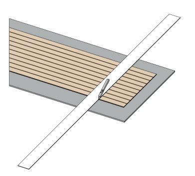
2. If the panels need to be cut to height, use the ThinRibbon knife with our ruler. To cut through the entire thickness of the panel, cut repeatedly in the same groove. Change the blade often.
