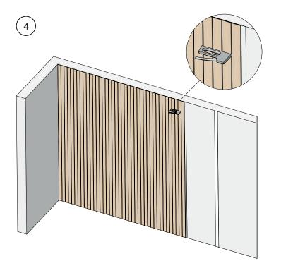
4. Using the ThinRibbon stapler, staple a few times into the black grooves to keep the panel in place during assembly.To install the next panel easily, check carefully that the panels reach the halfway point of the tape. Repeat this pattern.
